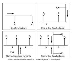
As their basis for fire flow testing of fire hydrants, PIAL uses the Main Capacity Flow Test process defined in NFPA 291, Recommended Practice for Fire Flow Testing and Marking of Hydrants, 2019 Edition – Chapter 4. This process requires there be at least two fire hydrants installed on the water main being tested. Use of a single hydrant for flow testing is only done as a last resort when there is only one serviceable hydrant on the main being assessed.
